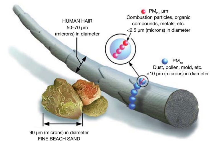
Figure 1. Schematic overview of the relative size of particulate pollution, PM 10 and PM 2.5
